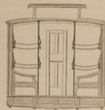
Fig. 8.—Transverse section of one of the hospital cars of the Army of the Potomac.—(Orrin.)
