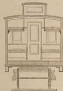
FIG. 5.—Transverse section of one of the hospital cars of the Army of the Cumberland.—(OTIS.)
