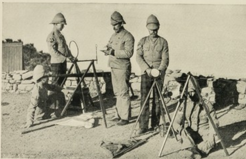
Transmitting a long-distance Message by Heliograph, Kasauli Signalling Station.
