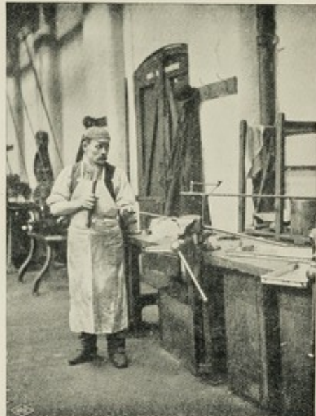
Boring a Barrel.
