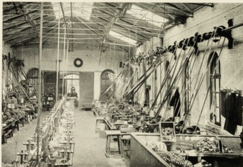
THE BAYONET ASSEMBLING SHOP. During the Dinner Hour, Here Bayonets are Put Together Complete.
