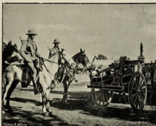
Photos. Copyright. AN INGENIOUS CONTRIVANCE. The Maxim Gun of Luncheon's Horse Mounted in a Transport Cart.
