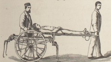
THE ASHFORD LITTER. THE STRETCHER DETACHED FROM THE WHEELED SUPPORT.
