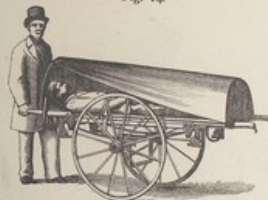
FURLEY'S ASHFORD LITTER. THE STRETCHER, WITH COVER, PLACED ON THE WHEELED SUPPORT.
