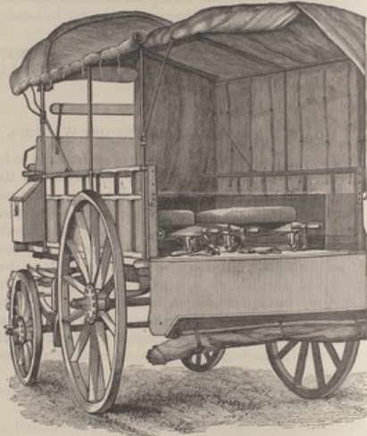
ENGLISH ARMY SICK-TRANSPORT WAGGON, SHOWING THE FARIS' STRETCHER RUN IN ON THE FLOOR OF THE WAGGON.—CENTRE BOARD NOT SHOWN IN ENGRAVING.
