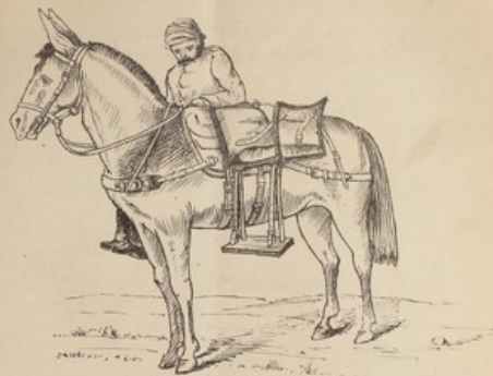
CACOLET FOR CARRYING WOUNDED MEN, Fitted with cushions, back and waist straps, slings and foot boards (weight 56lbs. per pair).
