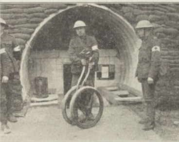
FIG. 6.—To show how compact the wheeled stretchers are when closed.
