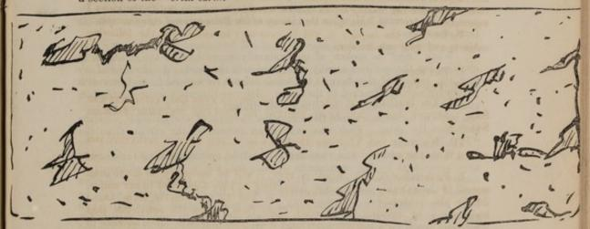
The shaded portions consisted of pure sand, and were more or less connected with each other in various directions. The intermediate structure was composed of fine clay and sand, combined in such proportions as allowed of percolation of water through their mass.
