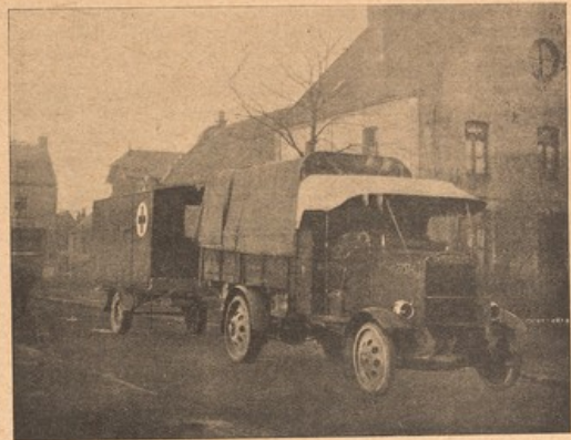
FIG. 1.—The Wallace-Cowell Theatre Trailer on the road, behind the tractor lorry. It follows readily wherever the lorry can go. Should the motor "break down" the trailer may be drawn to its destination by a pair of heavy draft horses hitched to either side of the traction pole.
