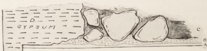
FIG. 9.—SECTION OF DOORWAY, THIRTEENTH MAGAZINE, KNOSSOS. A, fine plaster. B, rough backing. C, rubble wall. D, gypsum block with rebate for door.
