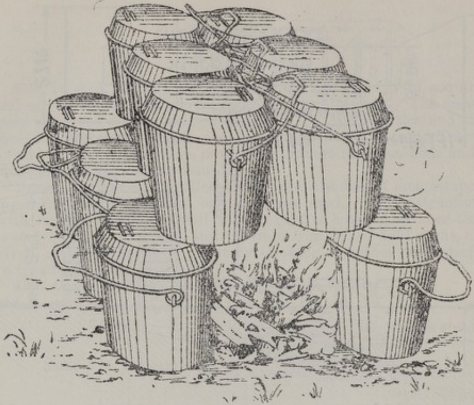
FIG. 94.—KITCHEN, WITHOUT A TRENCH WITH CAMP-KETTLES.
