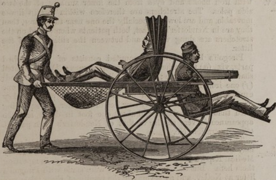
Fig. 1. —Neudörfer's Two-wheeled Litter, for the transport of one, or two, wounded soldiers.
