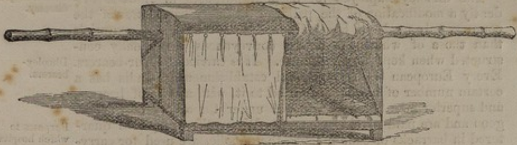
Fig. LX.—Bengal dhooley and bamboo pole complete, half of the side-curtain being thrown over the top in order to show the interior, with the mattress and pillow.
