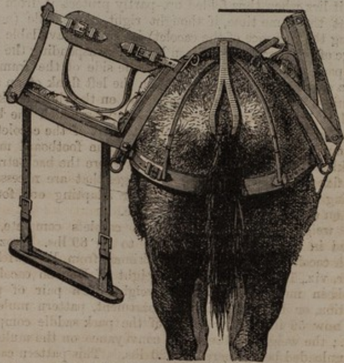
Fig. XCIX.—End view of mule chair or cacolet, open for use, and packed for travelling.
