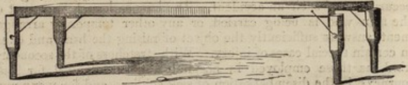
Fig. XXIV.—Side view of the same stretcher with its handles converted into feet.
