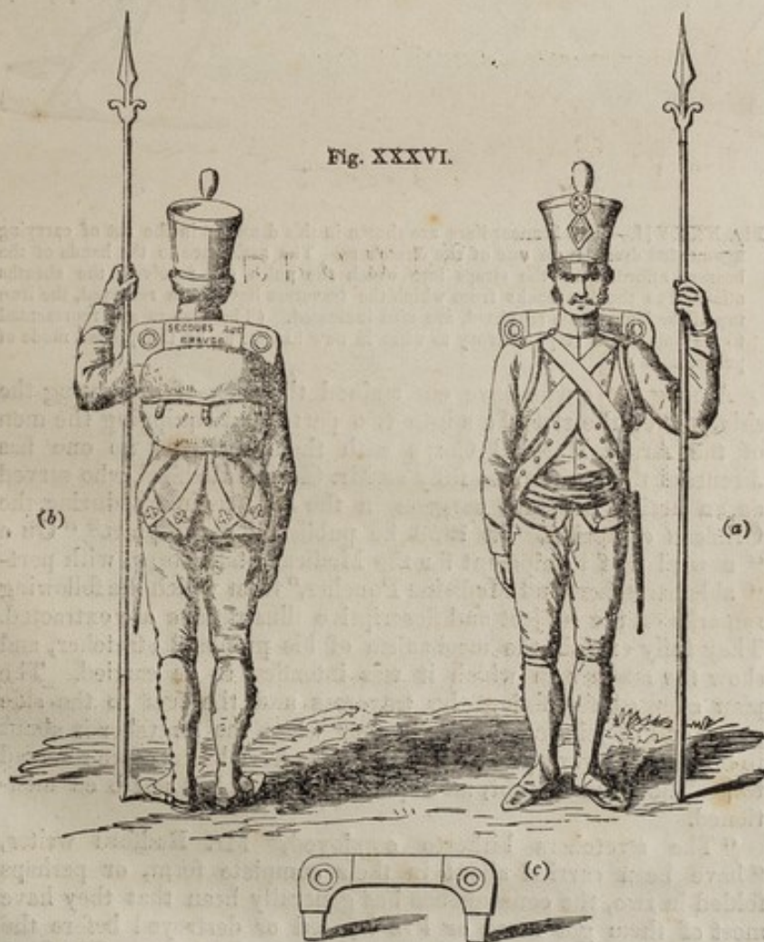
Fig. XXXVI.—(a.) Brancardier, equipped and armed. One of the traverses of the stretcher is carried upon the knapsack. Half the sacking of the stretcher is seen worn round the waist. The scabbard to receive the iron part of the lance when the latter is arranged for use as one of the stretcher poles is seen at the soldier's side.
