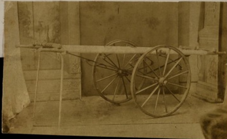
88 / Fig. A. — Shortell's Wheeled Stretcher-Support.—The springs are fixed upright by the action of the clamping screw in the nave of the wheel, which appears on the left of the drawing. The crutch pins are in the crutches.
