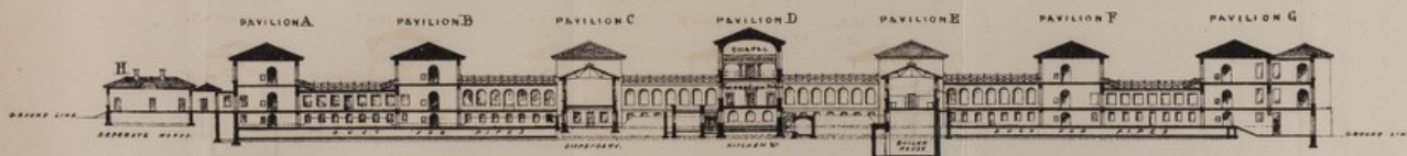
SECTION OF CORRIDOR SHEWING LEVELS OF BOILER-HOUSE, KITCHEN, &c.
