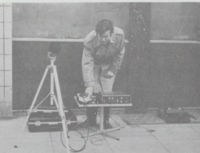
Measurement and recording of traffic at kerbside
