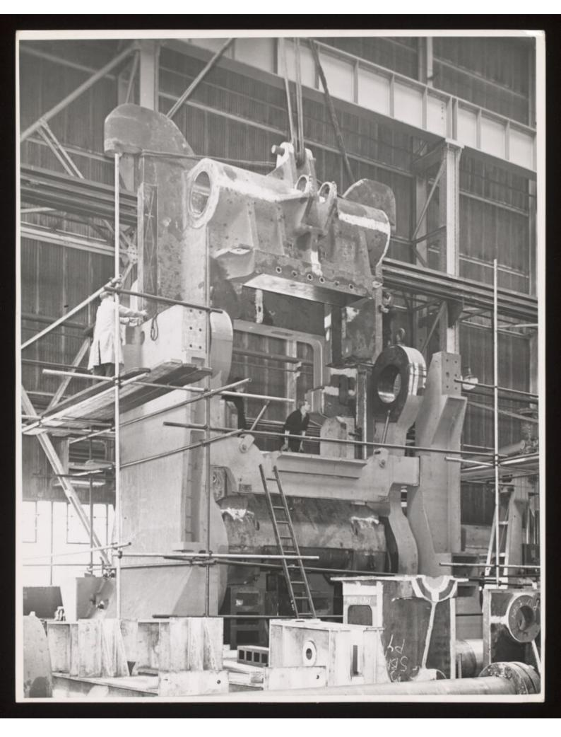
Engineering shop conditions in the firm of Davy and United Engineering Company, Ltd., Park Iron Works, Sheffield 4. One of a series of fourteen photographs supplied by Mr. F.R. Smith, Publicity Officer, 17th January, 1957. No. 4307. Heavy erection work for rolling mill engraving. The building of a 1350 tons hot bloom and slab shear embodying several single castings weighing around 50 tons each.
