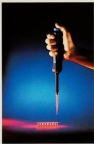
able, the Finnpipette Digital ACL has a number of other refinements. The softer body design achieves new levels in ergonomy to minimise hand fatique and arm strain during repeated use. The new tip ejector has been designed to ensure rapid clean detipping, particularly at volumes above 200µl where larger tips are used. Volume adjustment for each of the models is rapid and secure
