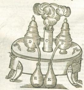
A Shews a brass Kettle full of Water. B The cover of the Kettle perforated in two places to give passage forth to the Vessels. C A Pipe or Chimney added to the Kettle, wherein the fire is contained to heat the water. D The Alembick confifting of his body and head. E The Receiver whereinto the diffilled liquor
