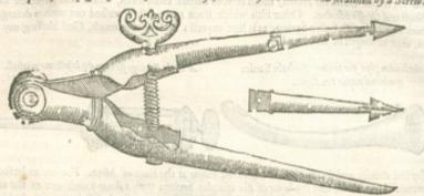
Moreover it is fit that the one leg of fach cutting Compaffes should stand firm and steddy, whilest the other is drawn circularly to cut. Wherefore it is fit you have an iron plate made full of little holes, wherein you may firmly flay that leg of the Compafs, left it waver against your will; it is requisite that this plate be crooked, (because the head is round) that so it may be fitted to any part thereof.
