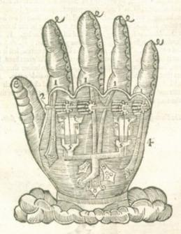
This Figure following showeth the back-fide of an Hand artificially made, and so that it may be tied to the arm or sleeve.
