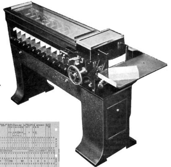
Figure 29: Hollerith card (left) and sorting machine (right), 1940s.
